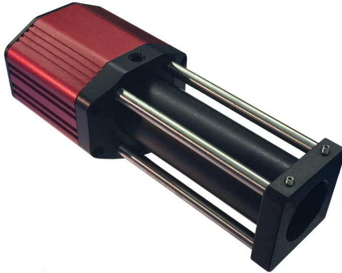
Figure 4 Camera Shown as Part of a 30 mm Thorlabs Cage System Using Ø1" Lens Tubes
